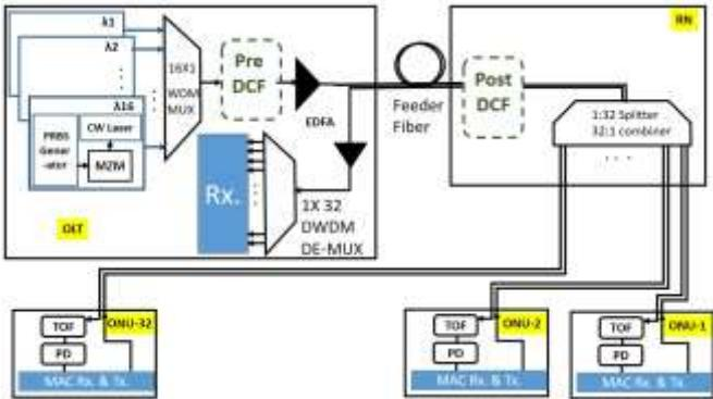
Fig. 1. Proposed architecture of WDM-DWDM-PON
