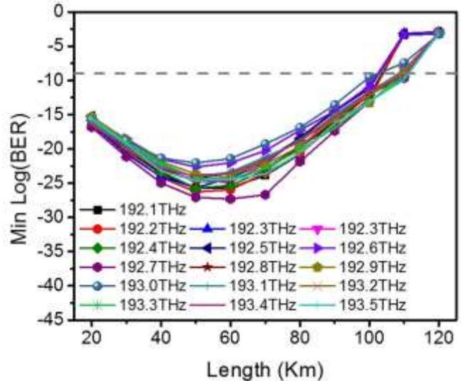
Fig. 8. Min Log (BER) vs reach of the fiber with pre dispersion compensation for every 16 wavelengths.
