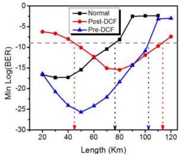
Fig. 9. Min Log (BER) vs reach of the fiber at 193.0THz frequency for uncompensated, post-compensated and pre dispersion compensated system architecture.
