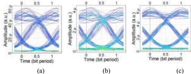
Fig. 10. Eye diagram of downstream channel 193.0THz for (a) Uncompensated wavelength at 70Km, (b) Post-DCF compensated wavelength at 110Km, (c) Pre-DCF compensated wavelength at 100Km.
