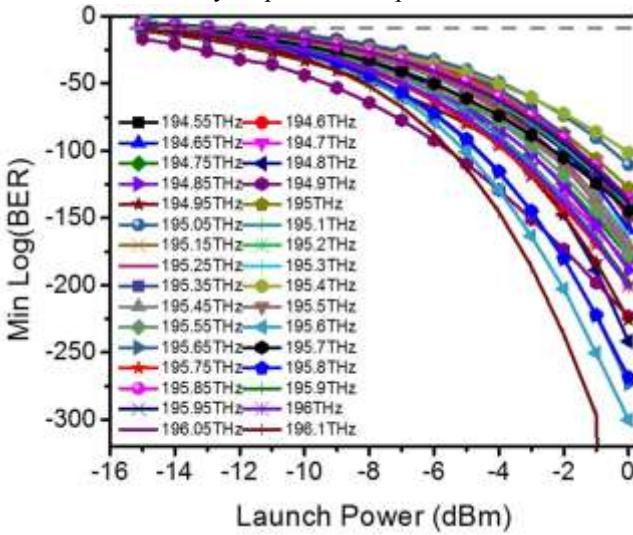
Fig. 3. Min Log (BER) vs laser launch power of each of 32 wavelengths
