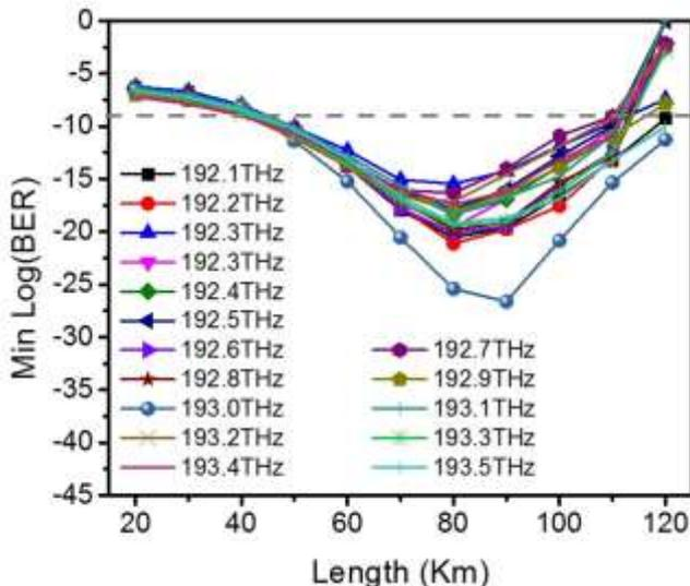
Fig. 7. Min Log (BER) vs reach of the fiber with post dispersion compensation for every 16 wavelengths.
