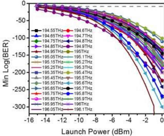
Fig. 3. Min Log (BER) vs laser launch power of each of 32 wavelengths
