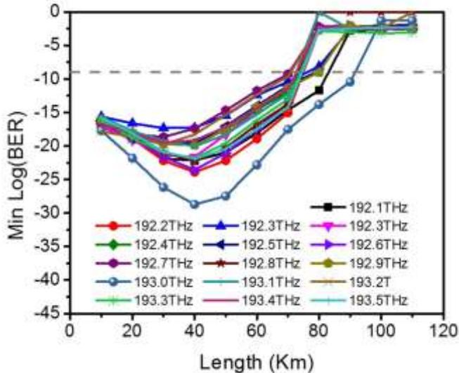
Fig. 6. Min Log (BER) vs reach of the fiber without dispersion compensation for every 16 wavelengths.
