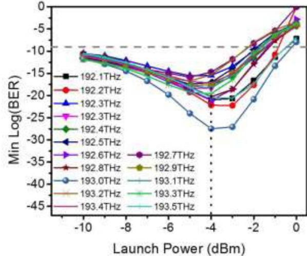
Fig. 5. Min Log (BER) vs laser launch power of each of 16 wavelengths
