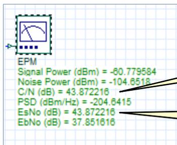
The C/N calculation here is for the total integrated signal power and noise power over 5 GHz BW. As the Signal and noise spectrum are relatively flat there is a close match between OSA measurements and the component calculation (43.8 dB)
